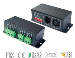
LT-DMX-6120 converts the universal standard DMX512 signal into SPI(TTL) digital signal to drive LEDs with compatible driving IC, it could control every channel of the LED lights, realize 0~100% dimming or editing all sorts of changing effect.
